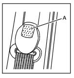
To move it up or down, press the square button (A) in the center of the height adjuster knob and move the height adjuster to the desired position.
